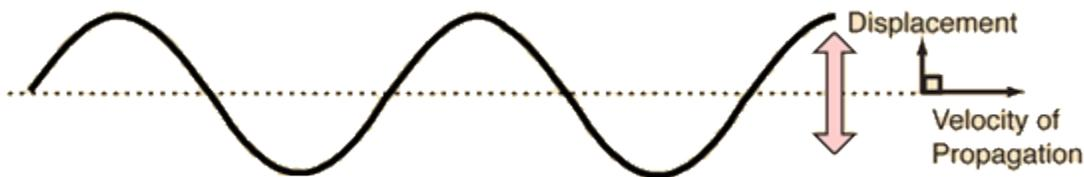
When a wave pulse (or continuous wave) reaches a boundary, or a transition, between two different media, there is a portion of the wave’s that will continue forward and be transmitted into the new medium. There is also a portion of the wave’s energy that will return back into the original medium (it is **reflected**).
