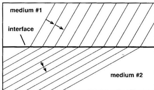
Figure 2.1: Refraction
